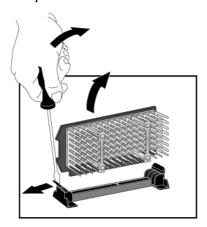
3 Install the new processor and clip it into place.
